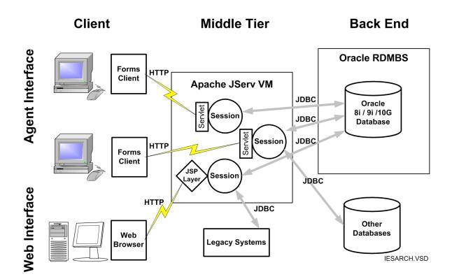
Using the Apache mid-tier architecture, business logic is executed on the enterprise Web server. The Apache JServ provides the Java Virtual Machine (JVM), executing the script at runtime as a servlet. Scripts are executed by the Scripting Engine using two different interfaces.
